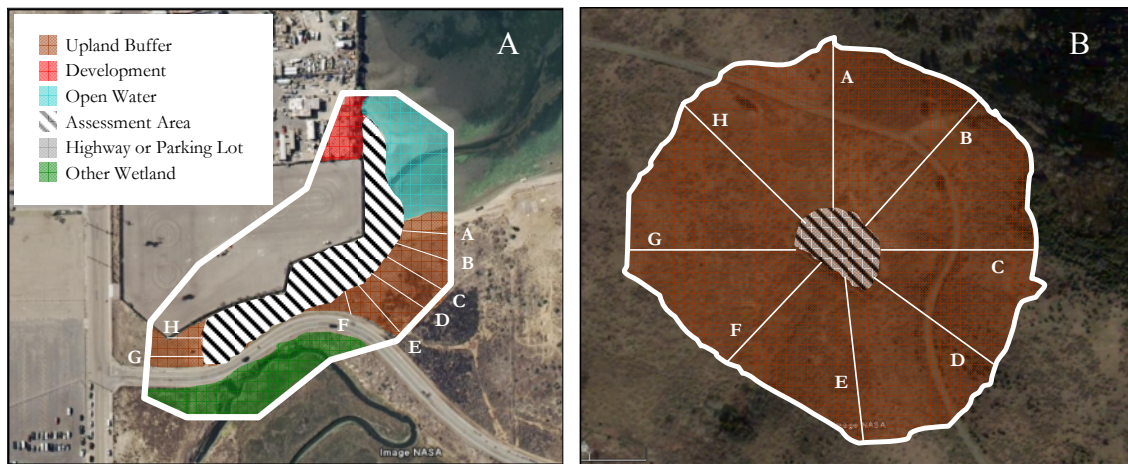
Figure 4.3: Examples of method used to estimate Buffer Width. It is based on the lengths of eight lines A-H that extend at regular intervals through the buffer areas, whether they are not extensive (A) or all encompassing (B).
