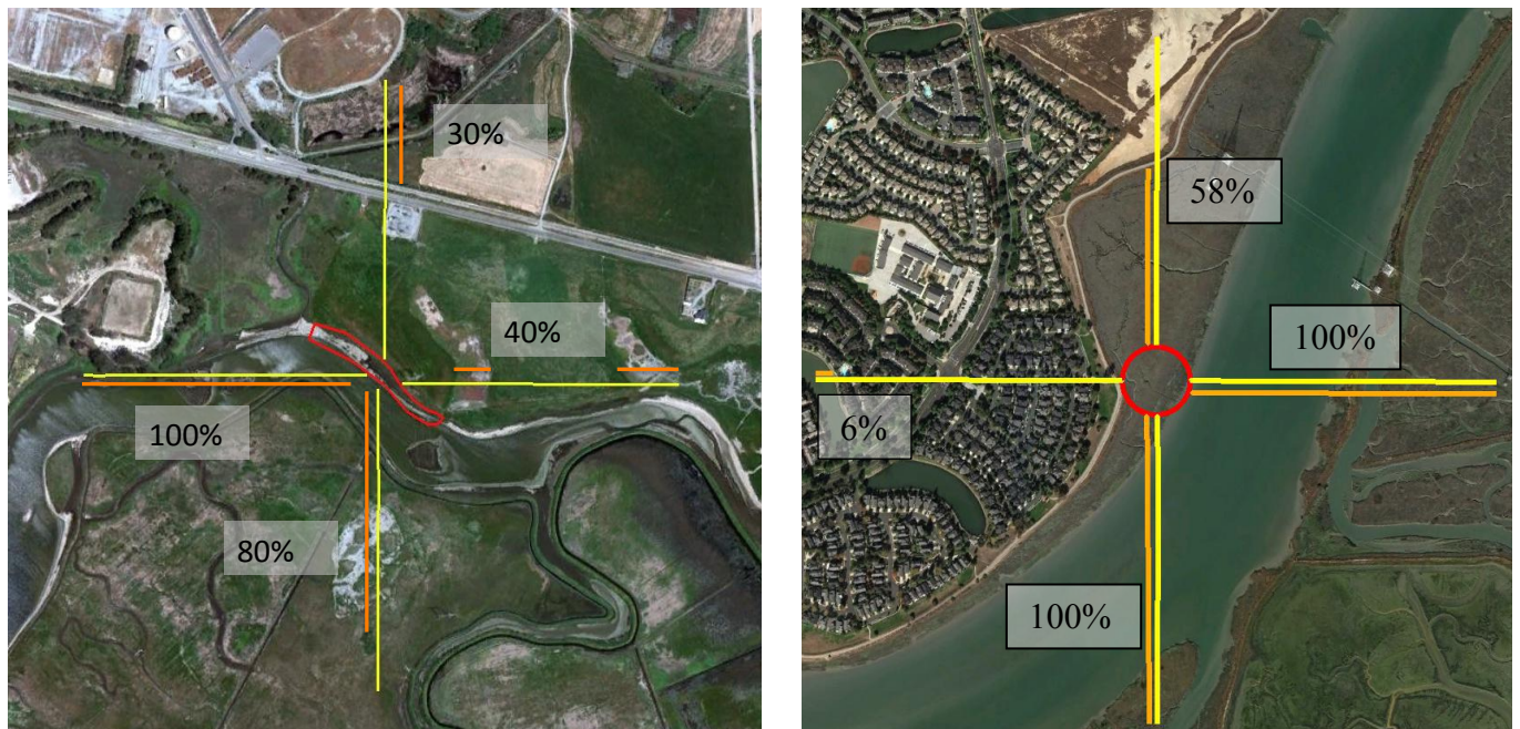
Figure 3: Diagram illustrating the method to assess the Aquatic Area Abundance of estuarine wetlands. The orange bars next to the yellow transect lines indicate portions of the line that pass through wetland or aquatic habitat. The first example shows that an average of 62.5% of the 500 m transects cross an aquatic feature of any kind. Note that this AA is positioned along a fringing estuarine marsh between open water and uplands. As a result, the AA is in a more linear shape. The second example shows a standard 1 Ha circular AA with an average of 66% wetland.
