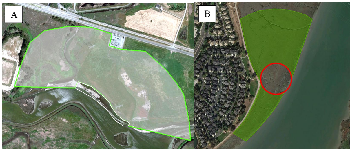
Figure 6: Diagram of approach to assess Buffer Condition for Estuarine AAs. In example A, the white line is the edge of the AA. Continuing with the example from above, this submetric assesses the condition of the buffer only where it was found to be present in the two previous steps (the shaded area with green edge shown). In example B, the buffer area is the shaded green region. The open water area is not considered in assessing buffer condition.
