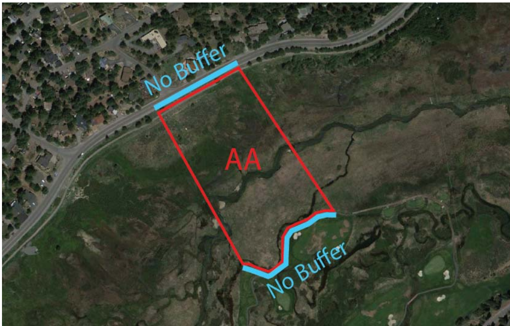
Figure 10: Diagrams of AAs with buffer and non-buffer land cover types. In the top example, the AA has approximately 85% buffer, with the road and the houses representing adjacent non-buffer land cover. In the lower example, the AA has approximately 65% buffer, with the road and the golf course representing adjacent non-buffer land cover.
