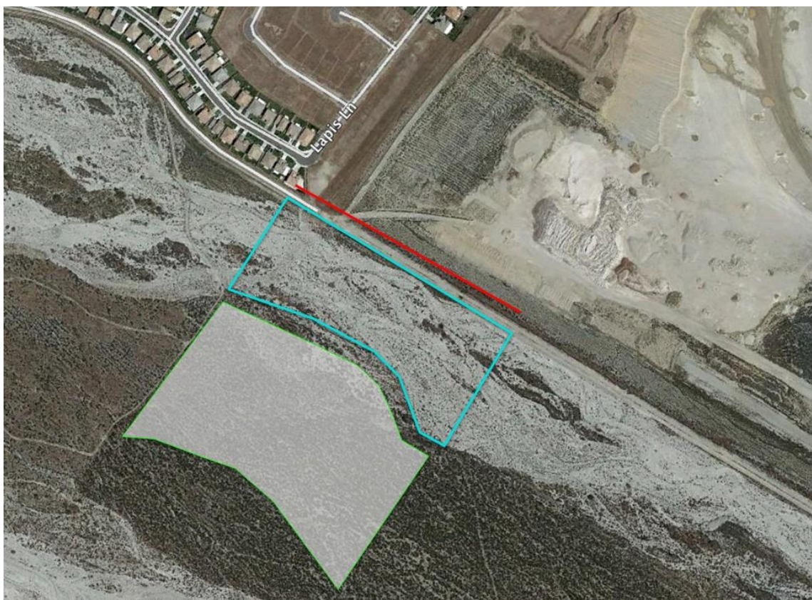
Figure 3.4: Diagram of method to assess Buffer Condition for Riverine AAs. Continuing with the example from above, this submetric assesses the condition of the buffer only where it was found to be present in the two previous steps (the shaded areas shown).
