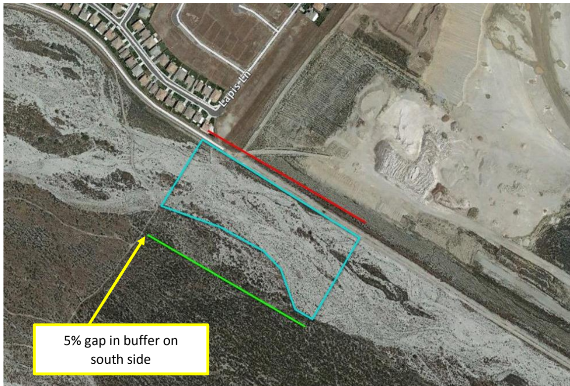
Figure 3.2: Percent of AA with Buffer for Episodic Riverine AAs. The blue line is the edge of the AA, the red line indicates where there is no buffer or less than 5 meters of buffer adjacent to the AA, while the green line indicates where buffer is present. The north side of the AA directly adjoins a non-buffer development, and on the southeast side of the AA there is a fence less than 5 meters from the AA. In this example 45% of the AA has buffer.
