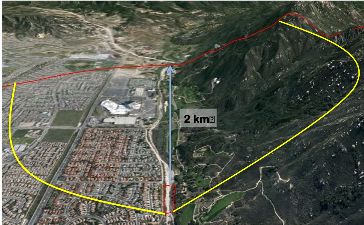
Figure 3.5: Diagram of approach to assess water sources affecting a CRAM AA showing an oblique view of the watershed. After identifying the portion of the aerial imagery that constitutes the contributing watershed region for the AA, assess the condition of the water source in a 2 km region (represented by yellow lines) upstream of the AA (represented with green box).
