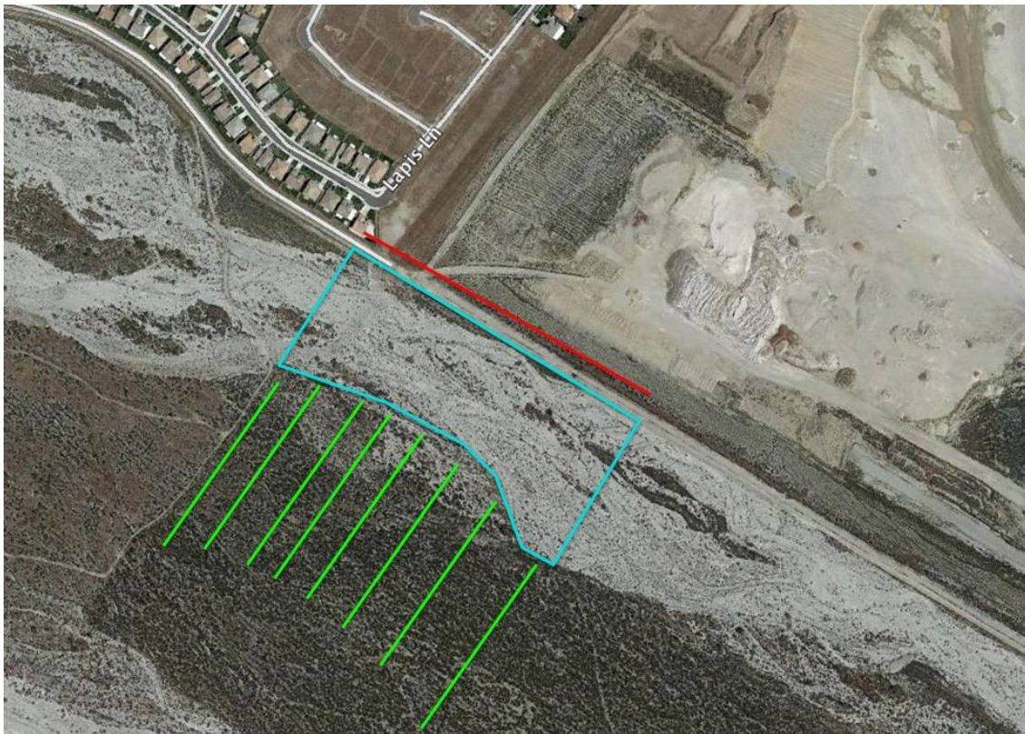
Figure 3.3: Diagram of approach to estimate Average Buffer Width for Episodic Riverine AAs. Continuing with the example from above, draw 8 lines evenly distributed within the buffer (red lines indicate where no buffer is present). The lines end in this example when they encounter the road to the south.
