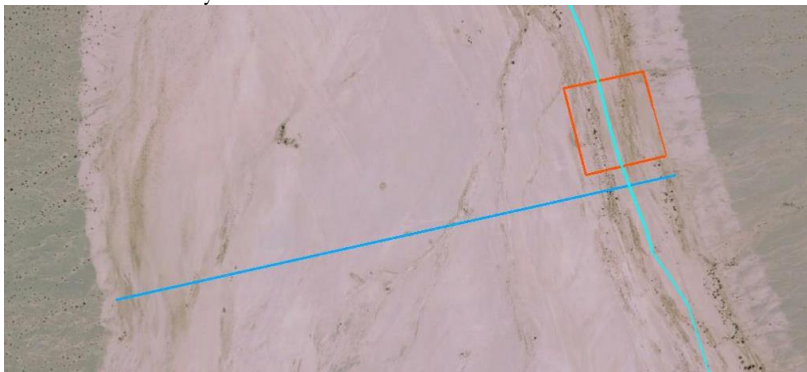
Figure 2.5. Diagram of episodic system with very wide floodplain. The light blue line represents the dominant low-flow channel. The dark blue line represents the active floodplain width (675 m). The orange box shows an appropriate AA with dimensions 200m x 200m.
