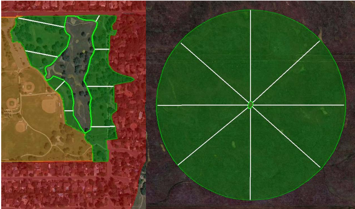
Figure 5: Examples of the method used to estimate Buffer Width. Note that the width is based on the lengths of eight lines A-H that extend at regular intervals through the buffer areas, whether only some of the 250 m zone around the AA is buffer (A) or all of the zone around the AA is buffer (B).
