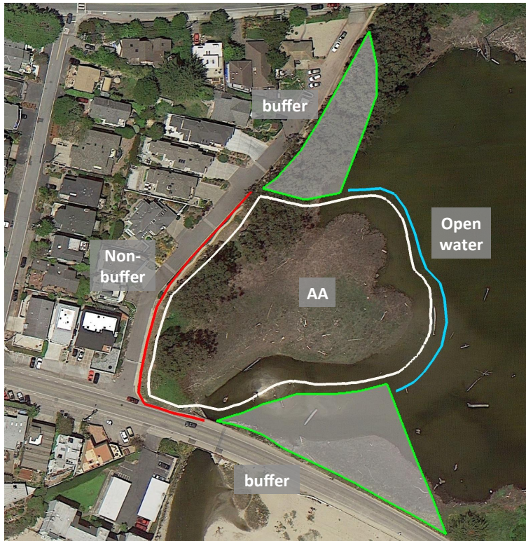
Figure 8. Example of buffer areas outside of the AA (white polygon) to be considered for assessment in the buffer condition metric for BBE wetlands (green shaded areas). Portions of the area directly adjacent to the AA that are open water (blue) and non-buffer landcover types (red) are not assessed.
