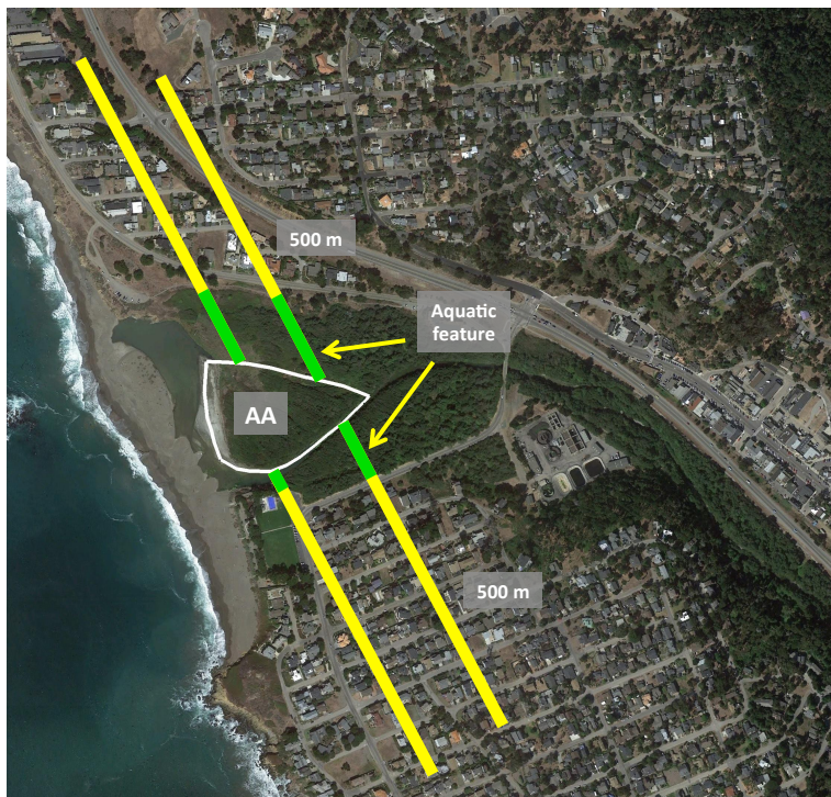
Figure 4. Diagram illustrating the method to assess the Adjacent Aquatic Area of BBE wetlands. The green portions of the 500 m yellow bars indicate portions of the line that pass through wetland or aquatic habitat. The example shows that an average of 20% of the four 500 m long transects cross an aquatic feature of any kind.
