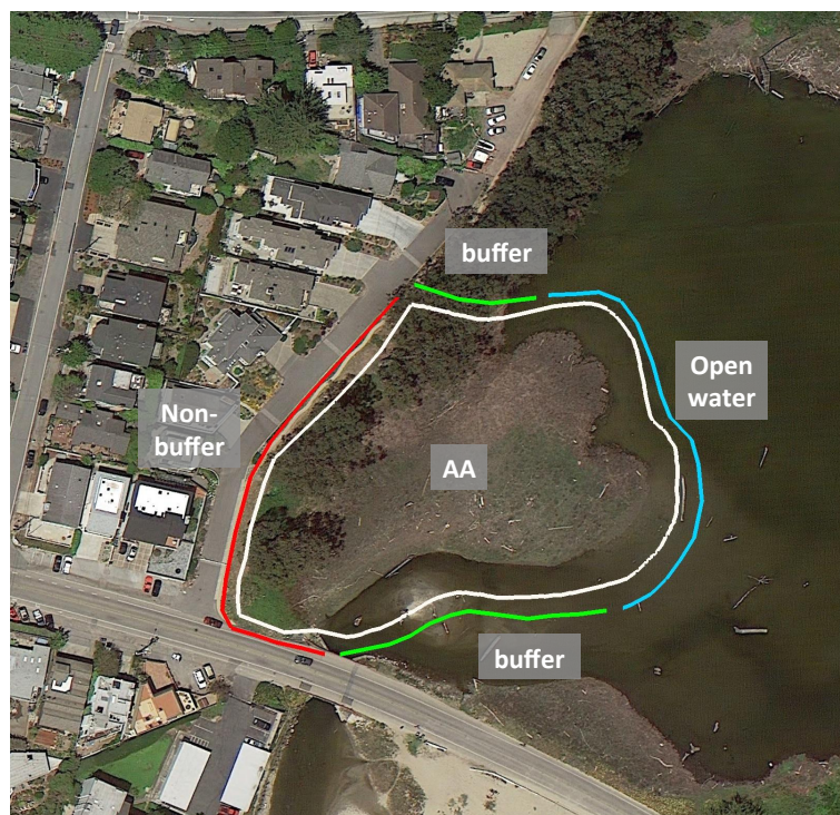
Figure 6: Diagram of buffer (green) and non-buffer (red) land cover types for a BBE assessment area (white polygon). The open water area (blue) adjoining the AA is neutral in the calculation of percent with buffer. Of the remaining perimeter of the AA, about 45% has buffer adjoining the AA that is at least 5 m wide. The non-buffer landcover types include roads and urban landscape.
